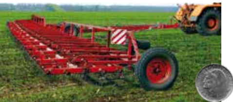
LIRA Hydraulic spring-tooth harrow
