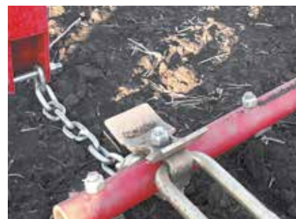
Adjustable attack angle
