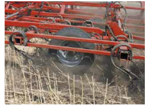
Cultivation depth adjustment
