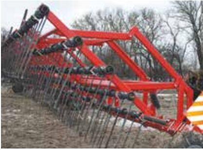
Suspension of working sections
