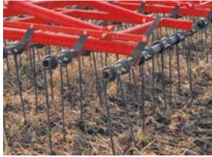
Adjustable attack angle
