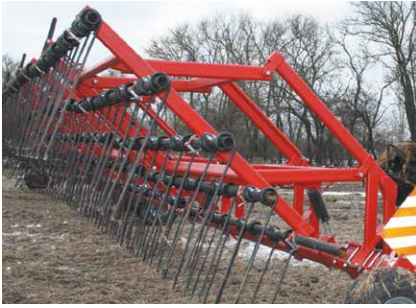
Suspension of work sections
