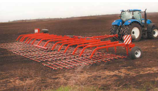
LARI Heavy tooth drag harrow and mineral fertilizers
