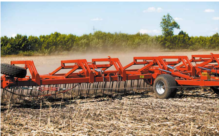
Cable tightening of sections
